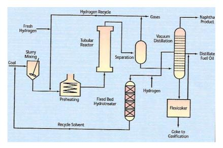
Figure 18 Schematic diagram of the EDS process (DTI 1999)
