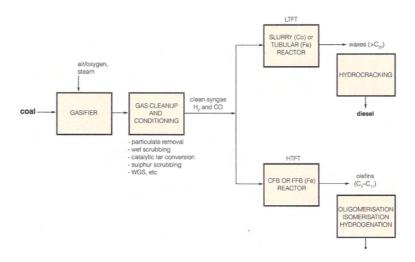
Figure 16 Process flow diagram for FT synthesis routes (Spath and Dayton 2003)
