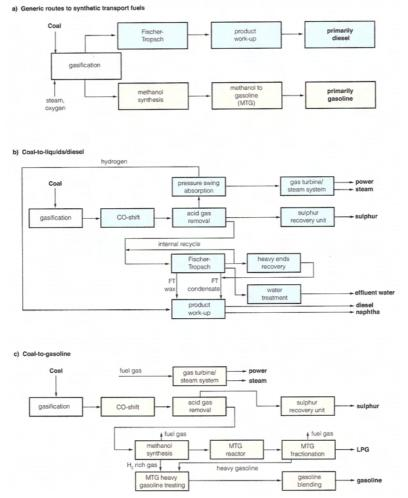
Figure 6 Flow diagram of the two generic routes to synthetic transport fuels using ICL (Radtke et al 2006)
