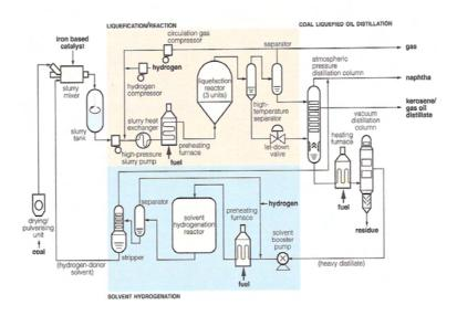
Figure 13 NEDOL process flowsheet for bituminous coal (NEDO, 2006)
