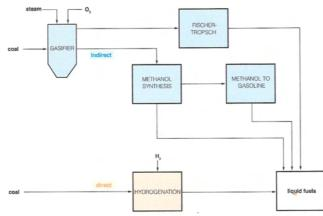
Figure 5 Principal process routes for the production of liquid fuels from coal (Couch 2008)
