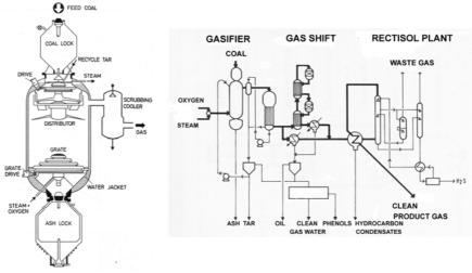
Figure A1 The Lurgi pressurised coal gasification process
