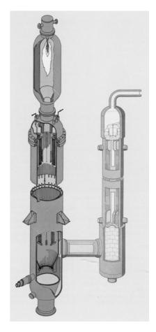
Figure A4 Prenflo Gasifier with radiation boiler
