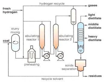
Figure 19 The CTSL two-stage process (DTI, 1999)
