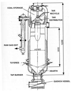
Figure A2 BGL Slagging Gasifier
