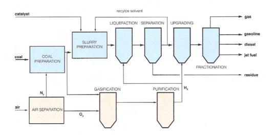
Figure 12 Shenhua DCL flowsheet for demonstration plant (Zhang 2007)
