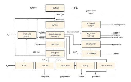
Figure 15 Process flowsheet for unit at Secunda (Steynberg 2005)
