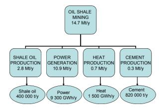
Figure 4 Material flows in the Estonian oil shale industry (Läänelaid 2009)
