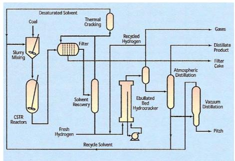
Figure 9 Schematic of the LSE process (DTI 1999)
