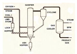
Figure A3 HTW process for fluidised bed gasification
