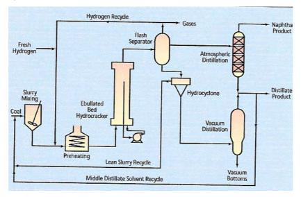
Figure 17 Schematic diagram of the H-Coal process (DTI 1999)
